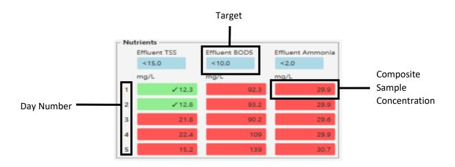
In order to score points, all 5 composite samples must meet the target (for one particular parameter, such as TSS). If the target is met for all 5 days, 100 points are scored. For example, all 5 TSS composite samples must be below 15 mg/L in the example above, and since the samples on days 3,4 and 5 do not meet the target, zero points would be score for TSS.
