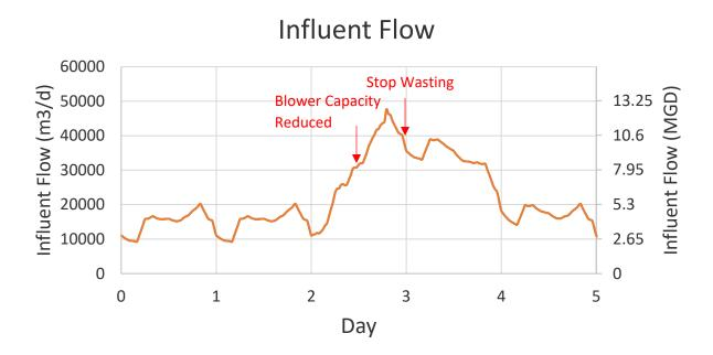
Note that a large wet weather event happens at the end of the 3<sup>rd</sup> day. All influent concentrations will be kept constant – only the flow rate changes over time. Also, the plant blower capacity is reduced to half and the wasting stops due to sludge disposal problem on the 3<sup>rd</sup> day, as marked on the graph above. In this question, one secondary clarifier is out of service for maintenance purpose and DO controller is unavailable for use.
